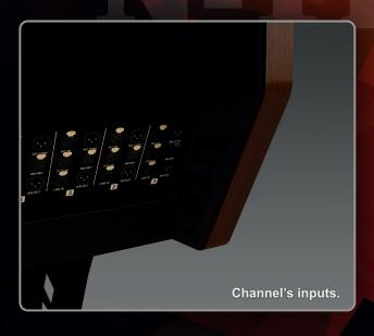
N-Trophy provides discrete connections for all channels, as well as for the Master Section. All of them are also available on patchbay. N-Trophy is the in-line console with independent MIC/Line and Tape inputs. Channel's sockets are:
